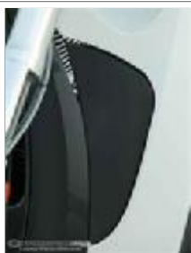
The 2012 Cross Country Tour comes with hard fairing lowers with vents that open and close to allow riders the ability to manage air flow. Here it is in the closed position.
